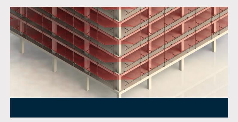
The SAFEDGE Safety Net Fan is a collective slab edge protection system for building construction to prevent or limit the fall of people and materials from height.
