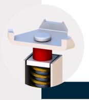
The spring mechanism allows the post to be compressed between the floor slabs and the vision gauge ensures that no full compression occurs.
