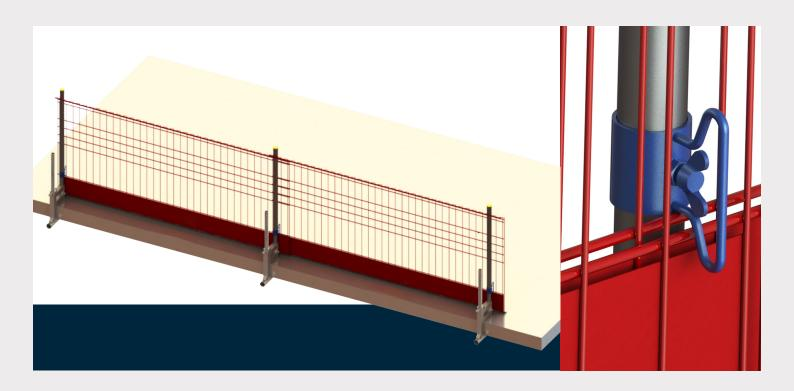
TG Slab Clamp System uses the same multi slab clamp as Safedge Clamp System. The Multi slab Clamp offers both horizontal and vertical clamping options and can be quickly set to a maximum of 450mm using the welded O.D 38 thread and tightened securely with a hammer.
