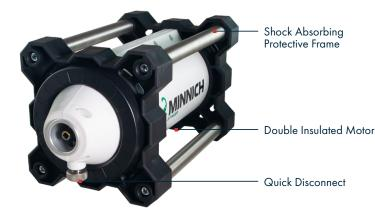
The Minnich Stinger is a 6.5kg electric flex shaft concrete vibrator. Like the Control Speed, the Stinger offers lightweight, durable, and versatile performance. Its universal motor operates at 15 amps (115-volt) and offers a compatible speed range of 11,000 to 13,000 vibrations per minute (VPM).
