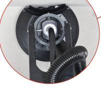
Fold up guard section for grinding edges.
